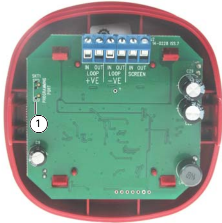
Fig. 4: Programming Port 1 – Programming Port
