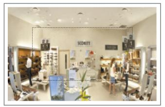
The dotted lines show the limited area covered by conventional PTZ cameras. If the man on the left was shoplifting, he would be out of view.
