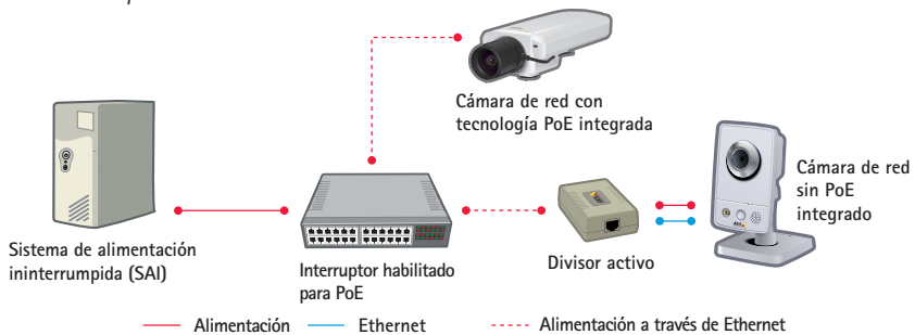
Figura 1.2b A system that uses Power over Ethernet.
