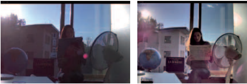
Figura 2.2d At left, image from a conventional camera. At right, image with a WDR camera.
