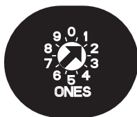
Figure 3.1: Address switch set to 1
