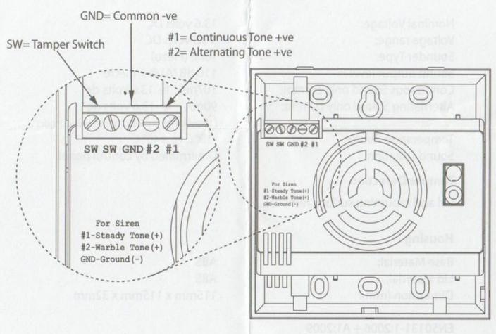
There are five terminals for the connection of wires as shown above. To activate either the alternating or continuous sound, connect a negative to the common negative terminal (GND) and connect a positive to the appropriate positive terminal (#1 or #2). To stop the sound, remove the positive or negative supply.
