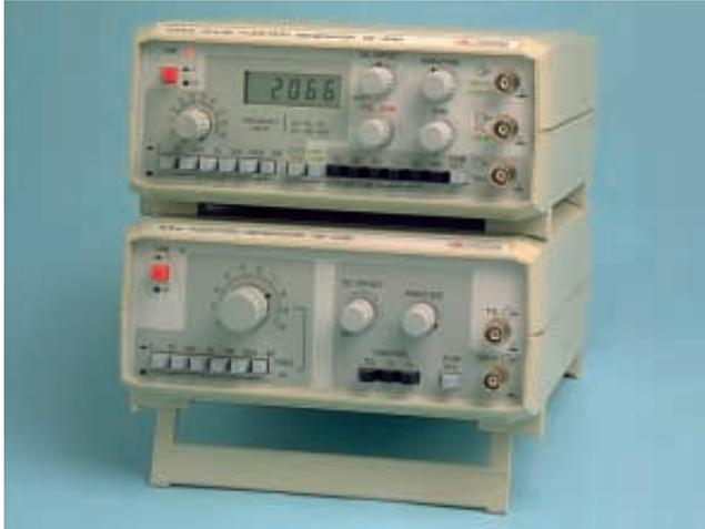
The GF-230 is a function generator covering the frequency range from 0.1Hz to 1MHz in seven decades. It allows to generate sinusoidal, square and triangular waves with continuous control of the output level, fixed 20 attenuator and the possibility to superimpose the signal at a continuous level through the DC OFFSET control. The VCO input located on the rear panel enables the user to control the output frequency and performs FM modulations to any auxiliary signal.
